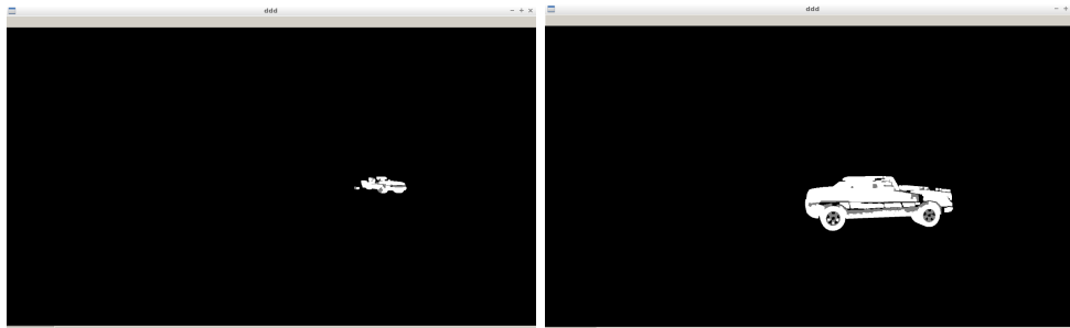
Figure 11: This is the output of the background subtraction procedure as the vehicle rounds the corner and passes in front of our agent.
